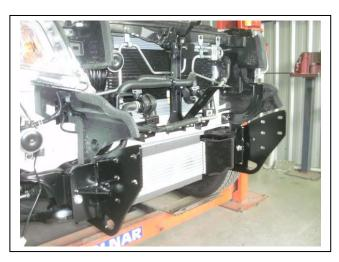
Figure 1: ECB steel mounts
