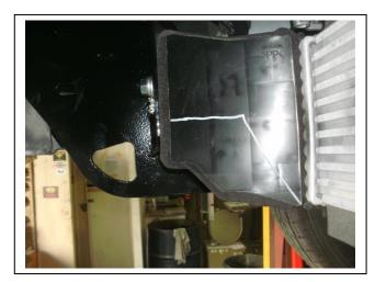
**Figure 6:** Intercooler air dam trim for under body guard fitment. Right hand side.
