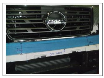
Figure 9: Mark 65mm down from grille as shown
