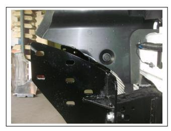
**Figure 4:** Left hand trim trimmed and installed. NOTE: the closer the trim the better.
