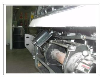
**Figure 3:** ECB winch mount with Mean Mother BOSS control box mounted
