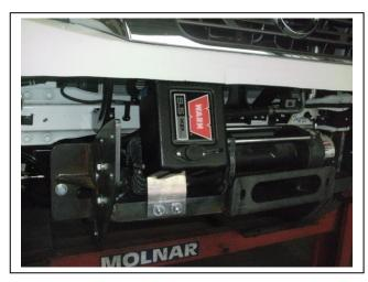
**Figure 2:** ECB winch mount with Warn 9.5 control box mounted
